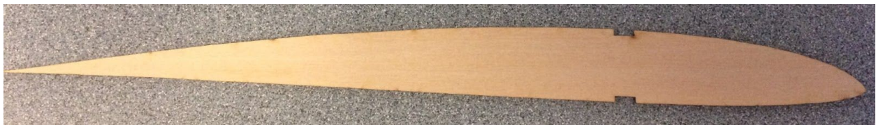
Figure 6.2.1: Laser Cut, Balsa Wood Rib
