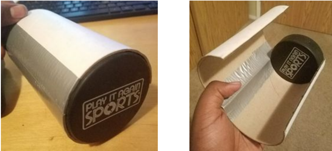
Figure 6.2.4: Payload canister (Without the Foam sealing)
